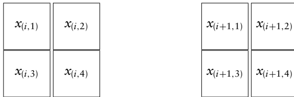
Figure 9.3. Part of a Pack network with four agents per pack. Each agent is connected to its three other pack mates, as well as the corresponding pack member in the next highest pack. Thus, agent x_{i,j} is connected to all of the other agents in pack i as well as agent x_{i+1,j} .
